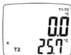
Every time the  $(T1-T2)$  button is pressed and held, the main/secondary display position of T1 and T2 will be switched. (TM-84/84D)
