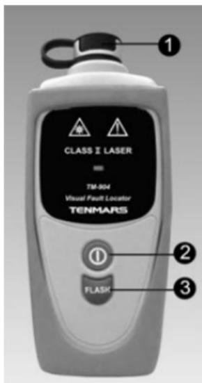
1. Remove off the dust cap and connect the fiber to the laser beam output port ① on the device.
