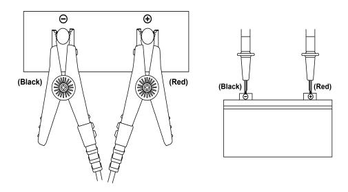
Read the battery internal impedance or DC voltage directly and Temperature measurement from the display.
