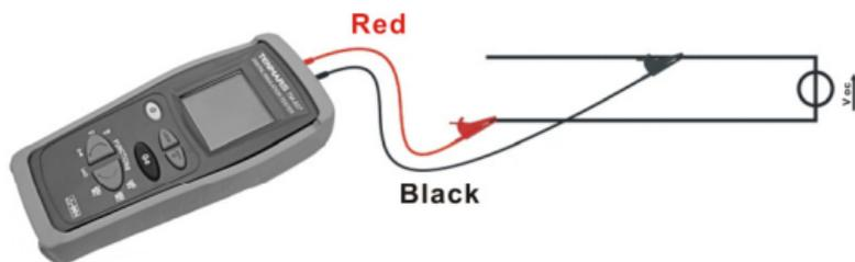
Connection of the instrument's terminals during
