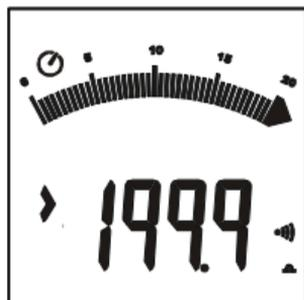
2. If the voltage present at the terminals is higher than 24V the instrument does not perform the test. The screen beside is displayed.
