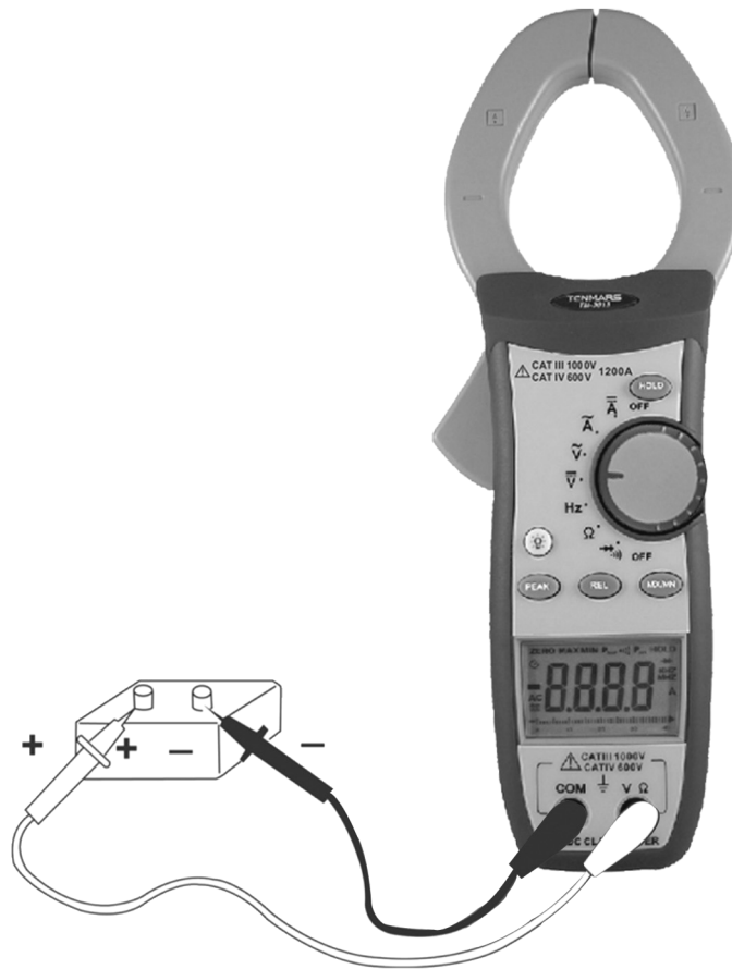
Fig. 6: Use of clamps for DC voltage measures
